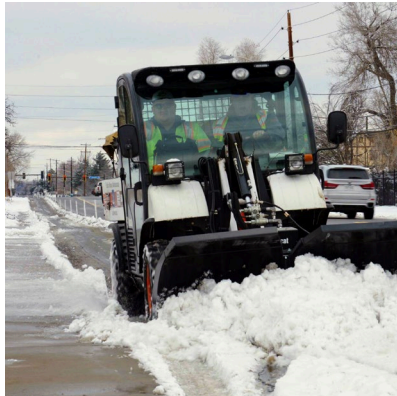
Figure 20: Scaled-down plowing equipment clears a separated bike lane.
