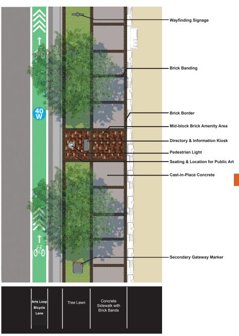
Figure 8: Brick and concrete streetscape concept
