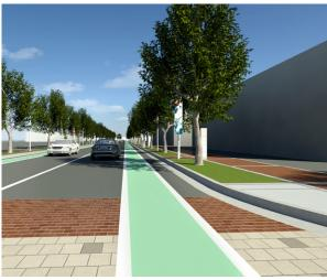
Figure 9: Lamar Street sidewalk, bike lane and pedestrian crossing concept
